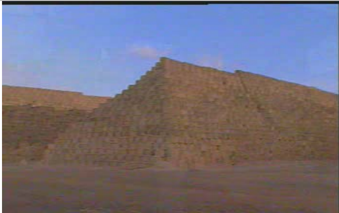
W -7. Heaps of bagasse cubes stacked for use in co-generation & paper production
